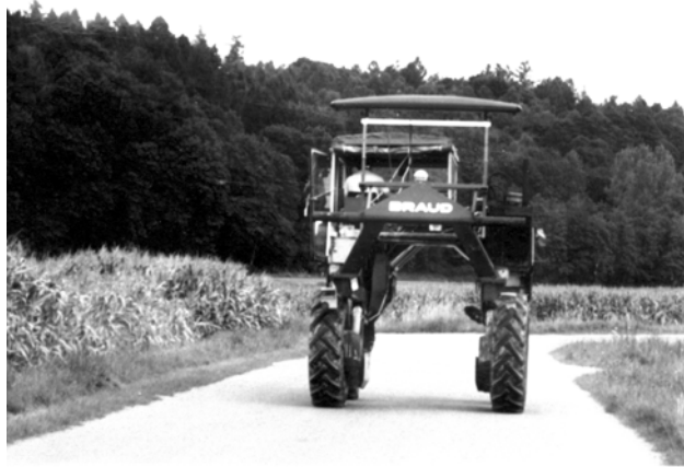
FIGURE 2. Crop scan sensor for measurements of biomass-/N-status mounted on a modified grape harvester for measurements in maize.
