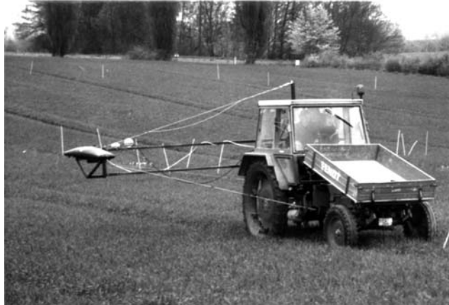
FIGURE 1. Crop scan sensor for measurements of biomass-N-status at reduced crop width mounted lateral onto a frame fixed to the tractor. The GPS is positioned on the frame to the right of the sensor.
