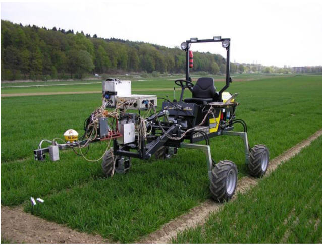
Fig. 1. PhenoTrac 4, measuring platform equipped with hyperspectral, thermal and laser distance sensors developed by the Chair of Plant Nutrition of the Technical University of Munich.
