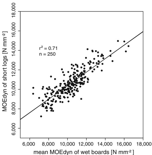
**Fig. 5** Relationship between MOEdyn of the short log and its wet boards sawn out of them; coefficient of determination  $r^2$  and sample size  $n$  of model 14 (Table 2)
