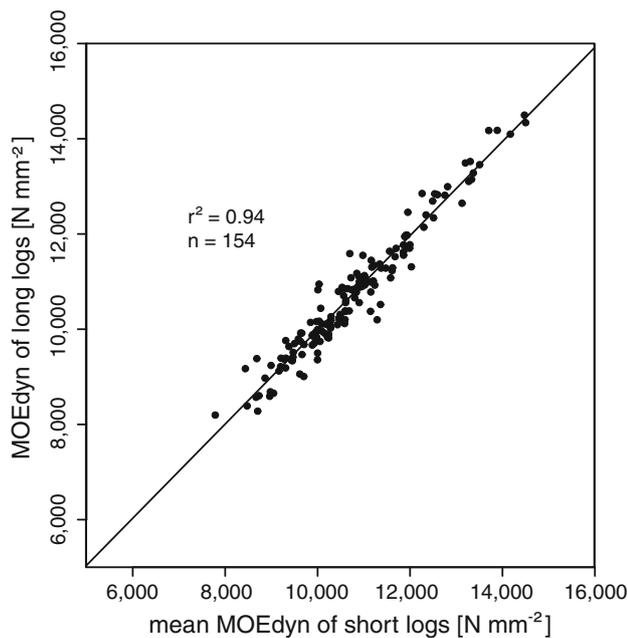
**Fig. 4** Relationship between MOEdyn of long logs and their short logs cut out of them; coefficient of determination  $r^2$  and sample size  $n$  of model 8 (Table 2)
