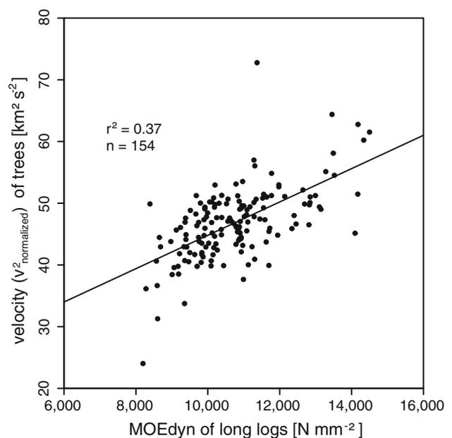
**Fig. 3** Relationship between wave velocity of standing trees and dynamic modulus of elasticity of long logs coefficient of determination  $r^2$  and sample size  $n$  of model 1 (Table 2)
