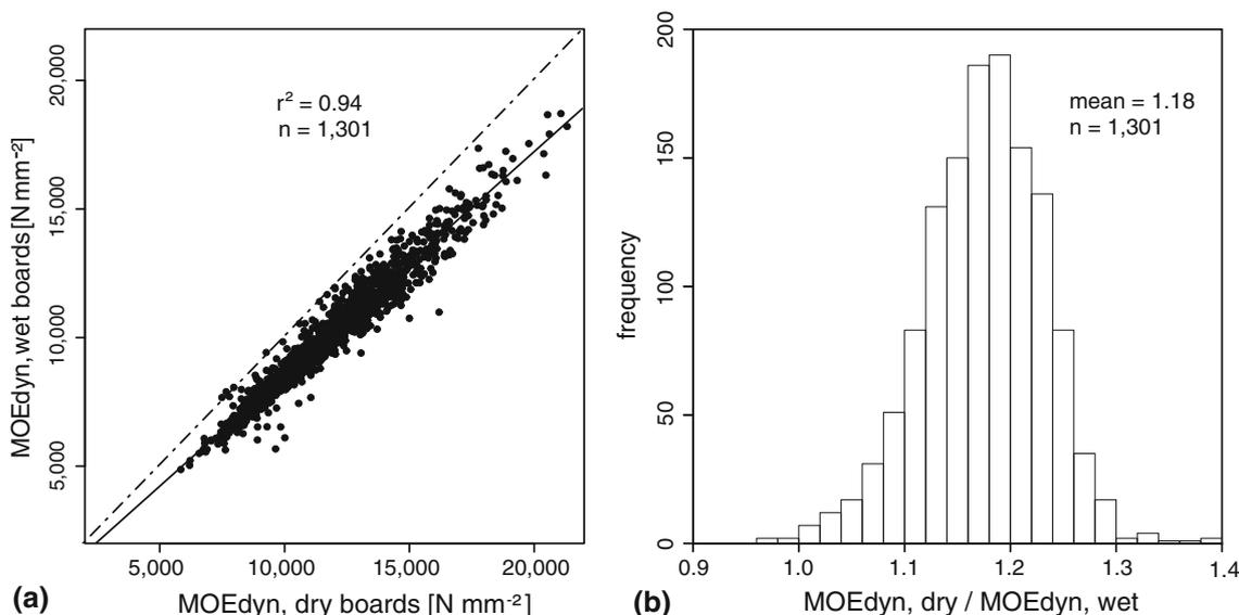
**Fig. 7** **a** Relationship between MOEdyn of dry and wet boards (model 23, Table 2); **b** distribution of the ratio between MOEdyn of dry boards and wet boards
