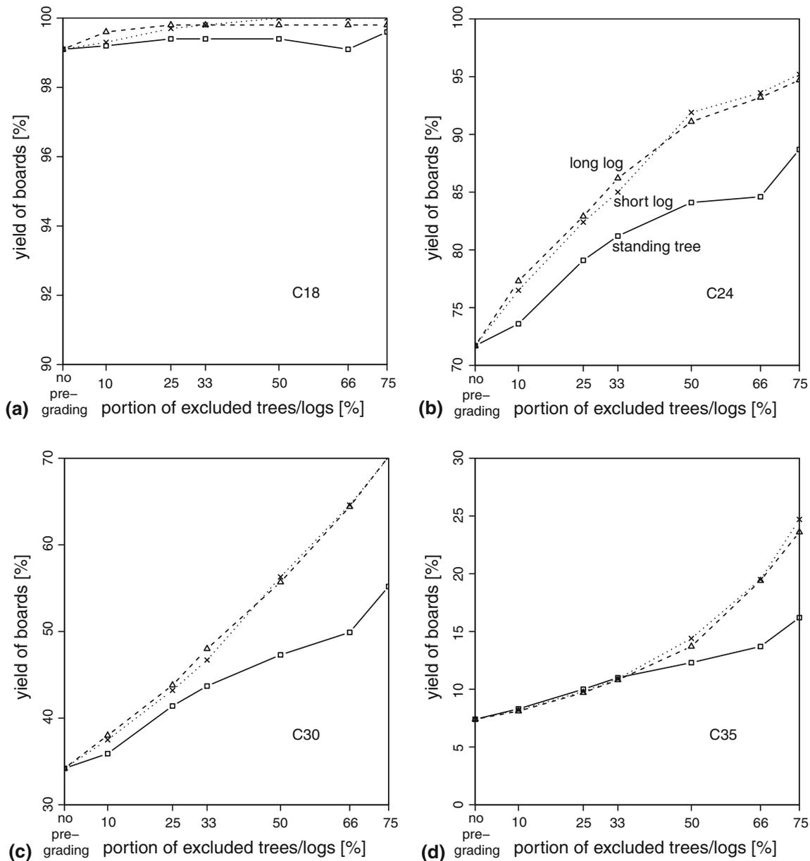
**Fig. 8** Increase of sawn timber yield with increasing portions of excluded logs—depending on level of pre-grading and strength class (a–d)
