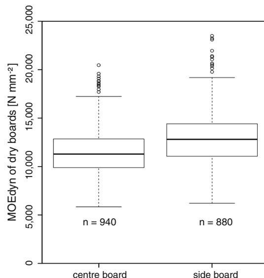
**Fig. 6** Difference of MOEdyn between centre and side boards is significant ( $p$ -value  $< 0.001$ ). The *box* defines 25 and 75 %-quantiles. The extent of the whiskers is 1.5 times the width of the *boxes* starting from the median
