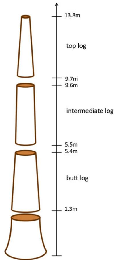
**Fig. 2** Each of the 154 long logs was crosscut to short logs of 4.1 m: butt, intermediate, and top log
