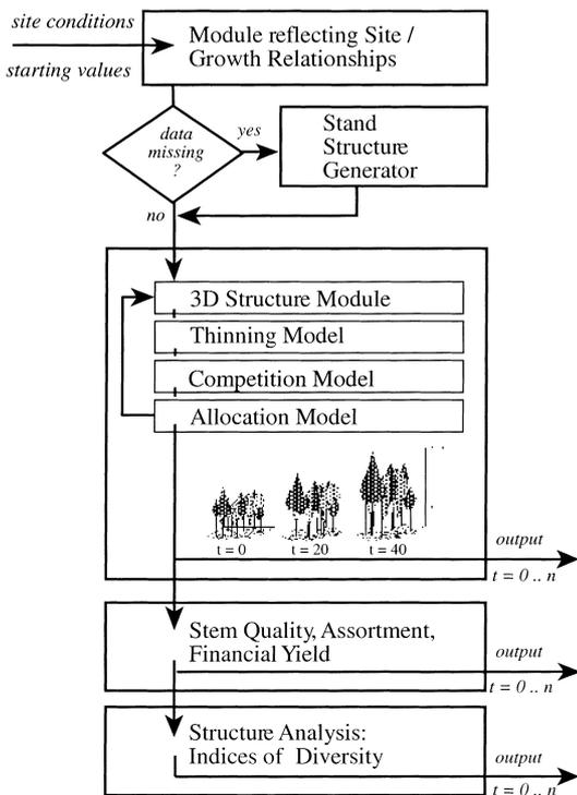
Fig. 3. The stand growth model SILVA 2.\* with the program module for structural analysis.
